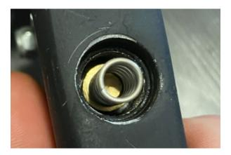
**Step #5** - replace the brass cap screw directly over the spring using a flat head screwdriver, tighten the brass nut cap screw until edges of brass nut screw are flush with inflator handle. **DO NOT OVERTIGHTEN.**
