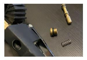
**Step #3** - insert the new brass plunger into the unit by pushing it all the way through the opening slot (flat end of plunger should be facing down)
