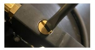
**Step #2** - remove the spring and push the brass plunger out of the unit
